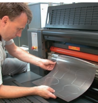
The inline die-cutting plate is fitted on the magnetic cylinder of the press.
